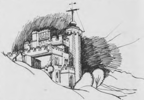
Lyttelton's Time Ball Station. Once a day the ball used to drop from the masthead to the base to give the port Greenwich time.
