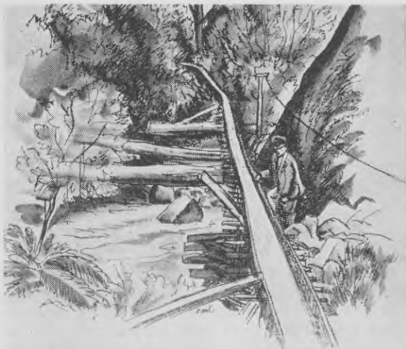
From the Cascade Mine the coal is "flumed" by water-power down a long trough for seven miles.
