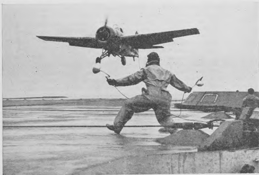
The deck landing officer guiding the pilot of an aircraft just about to land. This is done by means of "bats," which are reflectors containing lamps which can be seen easily.
