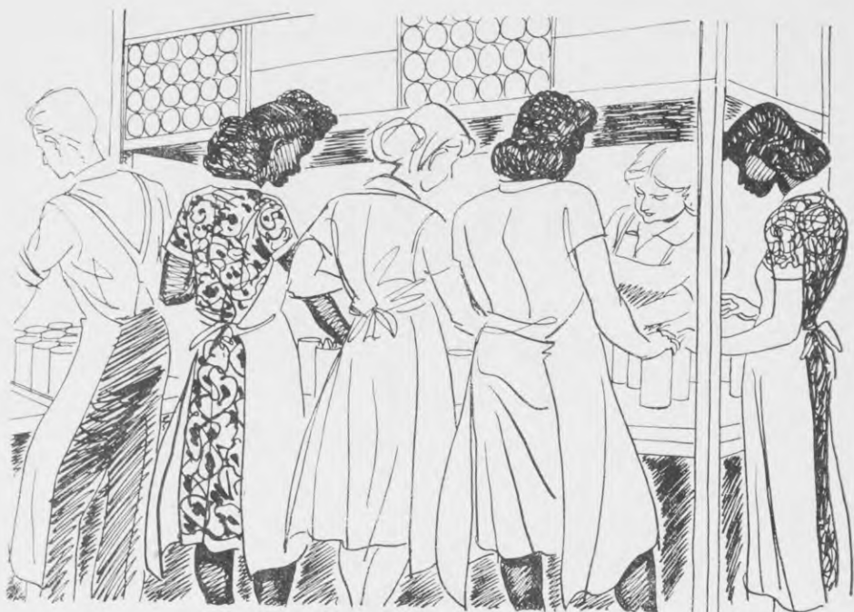
Filling the cans with cleaned fish. Empty tins are stacked above the girls. The filled cans pass down a travelling belt to the "crimping" machine, whose operator can be seen at the end of the table.
