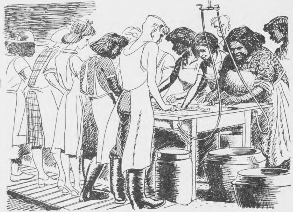
"Topping and tailing" the pilchards. The fish are taken from the mass in the middle of the table and, after being cleaned, are dropped into a water flume, which carries them down to wire baskets.
