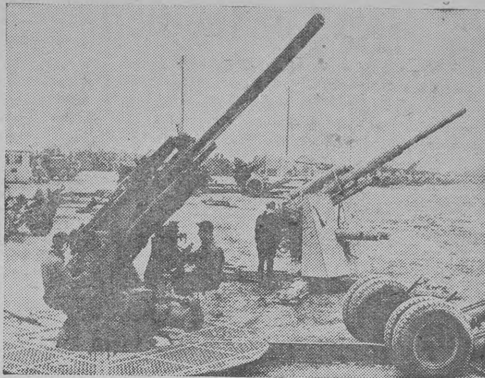
TESTING NAZI ACK-ACK GUNS—A captured German 88 mm. anti-aircraft gun (right) stands beside the corresponding American 90 mm. weapon. Exhaustive tests carried out at the U.S. ordnance proving grounds have shown the German gun inferior for both anti-aircraft and anti-tank work. The Nazis used the 88 mm. gun extensively in Africa.
