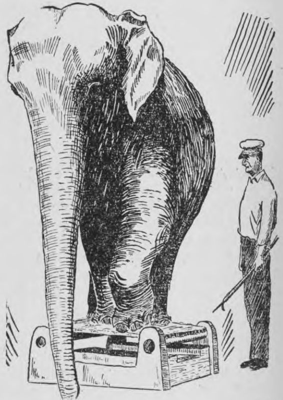
A plate of glass three-quarters of an inch thick can support the weight of an elephant with ease
