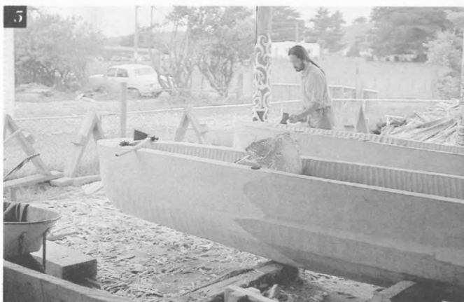
Kim adzes inner hull while older brother Greg adzes the other 1. Kim uses axe to block cut inner hull 2. Unpaid work team, Greg, Robert, Alan, Dave. Kim took the photo 3. Art of the adze. Greg remembers Kohe Webster teaching him adzing on an old power pole in 1976. Rua taught him in 1978 the broad blade adze art 4. Second hull bow shape 5.
