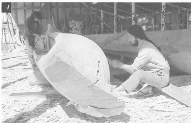
Kim adzes inner hull while older brother Greg adzes the other 1. Kim uses axe to block cut inner hull 2. Unpaid work team, Greg, Robert, Alan, Dave. Kim took the photo 3. Art of the adze. Greg remembers Kohe Webster teaching him adzing on an old power pole in 1976. Rua taught him in 1978 the broad blade adze art 4. Second hull bow shape 5.
