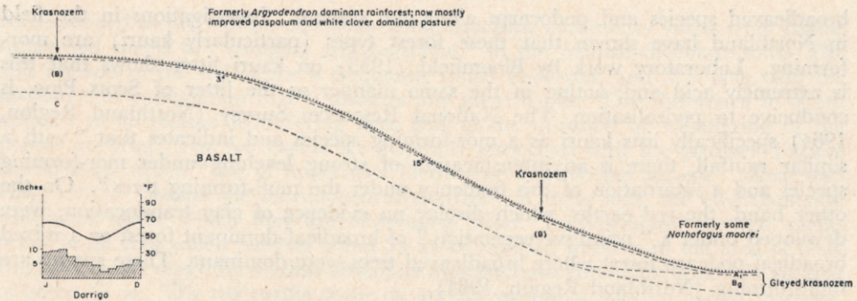
FIG. 5.—Dorrigo Plateau, N.S.W. Generalised catenary sequence of soils on basalt. Even higher rainfall at Dorrigo (inset) produces some gleying where there is interference from a ground-water table, but these soils otherwise have very little catenary differentiation.
