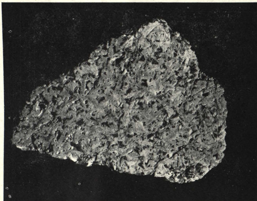
FIG. 2—Hand specimen of analysed syenite (length of specimen is three inches).
