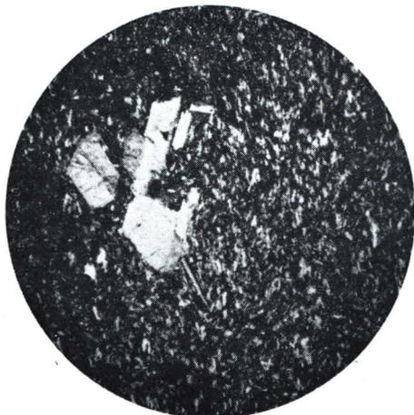
FIG. 2.—Keratophyre (2298). Small phenocrysts of albite in a trachytic groundmass. Crossed nicols,  $\times 15$ .
