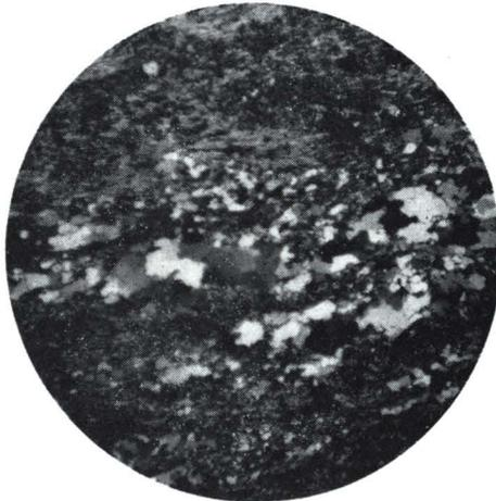
FIG. 3.—Quartz-muscovite-chlorite-epidote-schist (2185). Crossed nicols,  $\times 15$ .
