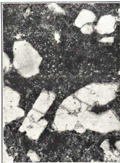
FIG. 4—Olivine phenocrysts set in a base of augite, iron-ore, and glass. P. 9150. \times 43 .
