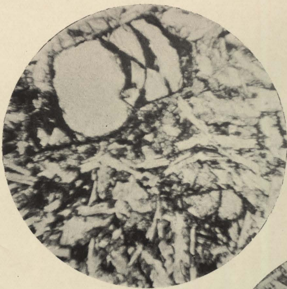
FIG. 17.—Basalt of a boulder on the west flank of Hunua Range. The photograph shows olivine serpenitized along fractures and around borders, laths of feldspar (white), and irregular crystals of augite (grey). The black material is partly serpentine and partly rod-like ilmenite. Ordinary light. Magnification, 45 diams.
