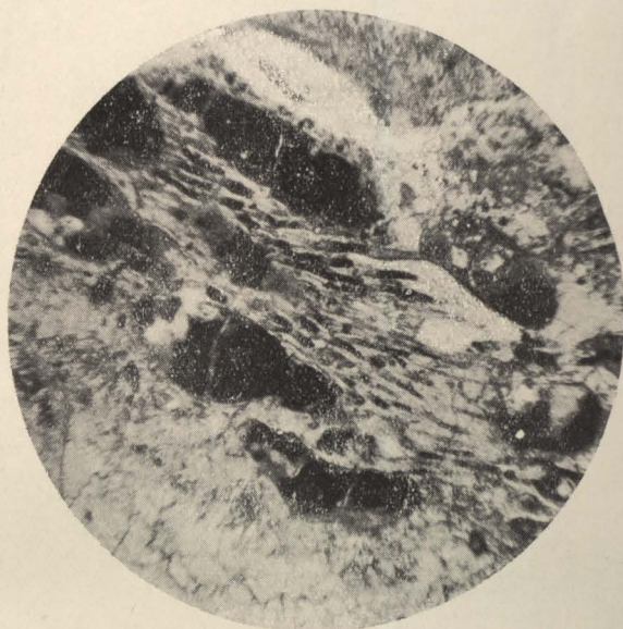
FIG. 14.—Longitudinal section of a polyzoan filled with glauconite. Papakura limestone, Bell Creek. Magnification, 45 diams.
