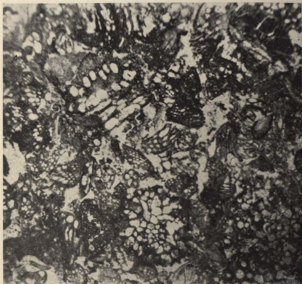
FIG. 16.—Typical section of Papakura limestone with abundant remains of polyzoa and occasional foraminifera. Magnification, 45 diams.
