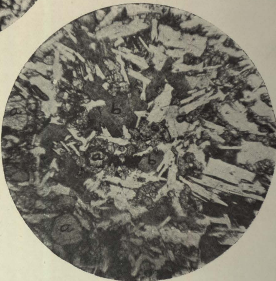
FIG. 18.—Basalt from the same locality as that of Fig. 17, showing irregular crystals of olivine (a), and augite (grey, high relief). Calcite (b) occupies interstices and is partly penetrated by laths of feldspar. Ordinary light. Magnification, 45 diams.
