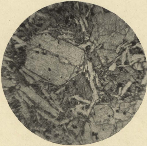
FIG. 37.—Coarse-grained basic olivine basalt, Green Hill Quarry. Large idiomorphic phenocrysts of olivine appear in groundmass of augite, plagioclase and magnetite. Ordinary light; magnification, 46 diams.
