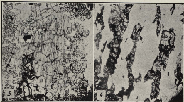
FIG. 5.—Diopside-garnet-gneiss, No. 4694. Diopside at centre (showing cleavage) surrounded at sides of photograph by garnet and interstitial quartz. FIG. 6.—Diopside-hypersthene-gneiss, No. 4687. The colourless clear mineral is plagioclase.
