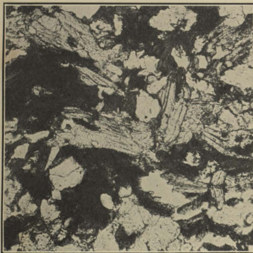
FIG. 3.— Coarse-grained gneiss (No. 1278), with plentiful biotite and muscovite, quartz, and andesine.
