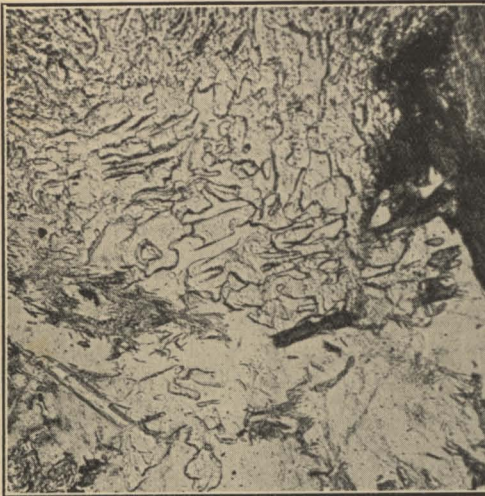
FIG. 5.—Intergrowth of quartz and muscovite in coarse-grained composite gneiss (No. 1338a).
