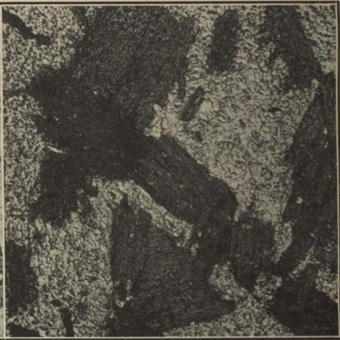
FIG. 8.—Micaceous band in porphyroblastic hornfelsic paragneiss (No. 1345). Large sieved crystals of biotite are enclosed in a fine-grained groundmass of muscovite and quartz.
