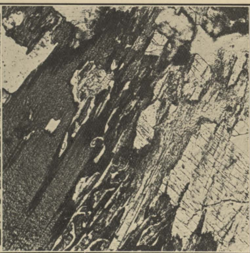
FIG. 4.— Intergrowth of vermicular quartz and biotite in coarse-grained composite gneiss (No. 1338a), Note also the partial replacement of the large crystal of feldspar by sericitic mica.
