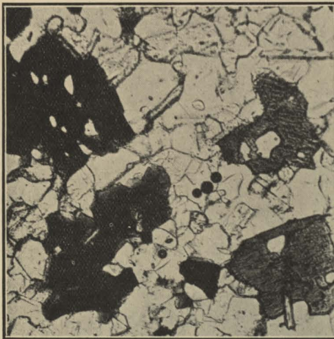
FIG. 7.—Porphyroblastic hornfelsic paragneiss (No. 1349), showing large crystals of biotite sieved with small inclusions of quartz and muscovite.
