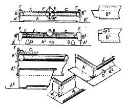
overlapped and interlaced, and the top, or any two corners, secured by special bolts from one member to the other. A further feature lies in the combination of the roll top with part of the wall of the main frame, strengthened at the lower edges, with the remainder of the wall of the main frame strengthened at the upper edges.
