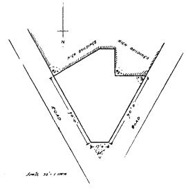
It is desired that the banking chamber shall extend as nearly as possible the full width of the site, and also that the same shall be symmetrical. In this instance a corner entrance must be arranged for, and no columns or piers are to occupy the floor space of the chamber.
