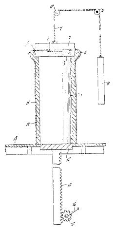
completed the head is removed by means of a chain passing over a pulley. The body part of the mandrel is then lowered through the floor by means of a rack and pinion. The periphery of the head has swellings for forming the faucet.
