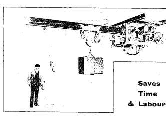
ALL OPERATIONS BY MOVEMENT OF ONE HANDLE. DRIVEN BY BELT, ROPE, OR MOTOR
