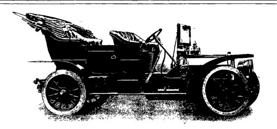
THE F.I.A.T. Cat, 15/20 h.p., 4-cylinder, complete with Hood, Screen Side Lamps, Tail Lamp, Horn, Kit of Tools, Pump, Jack, Tyre Repair Outfit. 2775
