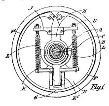
lug (E1), and (K) a similar bar formed on the wedge (H). These cross bars are connected by springs (L), and have a tendency to force the wedge between the friction rollers on the arms (F, F1). A bell crank lever (M) engages the sliding wedge and is engaged by a sliding collar (N), operated by a clutch fork. When the collar is moved towards the clutch,
