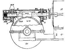
The ball races (S) are stationary and attached to the bearing (B), whilst the revolving races (R R) are attached to the shaft. The thrust is transmitted by the collars (c), and the pull by the lock nuts (n), to their respective ball bearings, thence to the solid bearing (B), and by means of the flanges (f) to the gear case.
