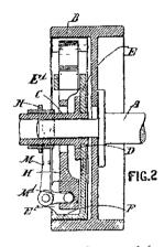
the wedge (H) is drawn down and frees the spring arms so that they are out of engagement with the clutch drum, and when the collar (N) is released the springs force the wedge between the ends of the arms and cause them to engage with the drum
