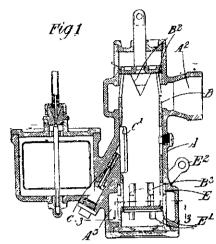
base of the sleeve are other apertures (B3) which co-operate with openings (E1) in a ring (E) surrounding the lower end of the tube. The ring (E) lies in an annular space (A3) in communication with the atmosphere by an inlet (A1), and can be
