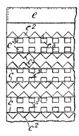
surfaces (c, c) are formed from stampings of sheet metal bent into trough-shaped form and having flanges (c2) preferably serrated, and apertures (c3) The gills not only act as distance pieces between
