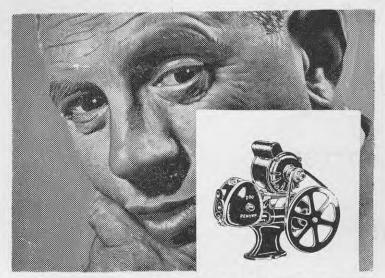
Renowned as the height of efficiency in the water pump field. CAPACITY: 200 gallons per hour at 255 R.P.M. with a maximum head of 150 ft. or 65 lbs. Also available is the "twin" Renown "400" pump.
