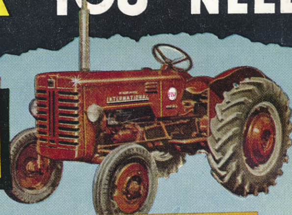
The outstanding McCormick International B-250 30 H.P. DIESEL TRACTOR DIFFERENTIAL LOCK DISC BRAKES
