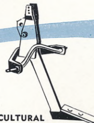
GL-224 AGRICULTURAL RIPPER For hard ripping to 16ins. below ground level. Easily adjustable and tipped with silicone manganese steel.
