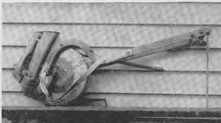
This type of depth-limiting skid when fitted to a disc-coultter drill prevents excessive penetration in soft patches while allowing full spring pressure to be applied. Thus an even-depth furrow is assured.
