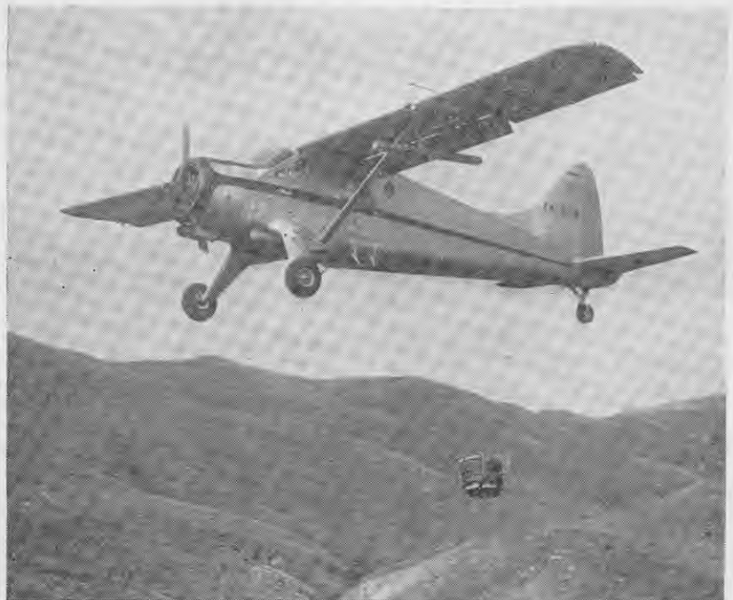
▼ Dropping a load of four coils of wire on a drum and steel posts. Aerial dropping of fencing material on hill country has a great future.
