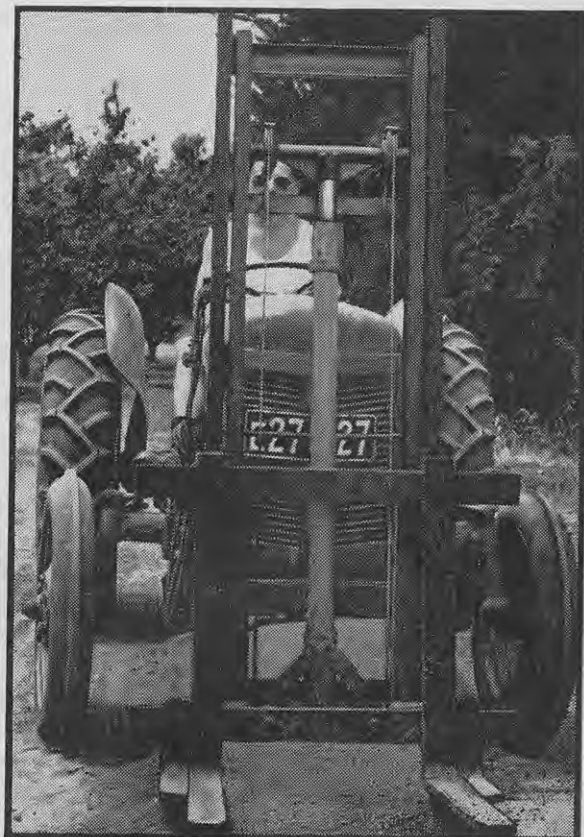
Above—Side view showing method of attaching the lift to steam piping supports, which extend the full length of the tractor. Below—Front view showing hydraulic ram and construction of main framework.
