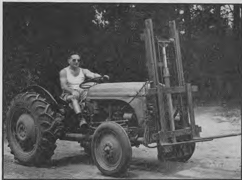
Above—Side view showing method of attaching the lift to steam piping supports, which extend the full length of the tractor. Below—Front view showing hydraulic ram and construction of main framework.
