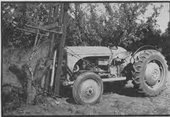
The attachment can be put to many different uses. Above—Pulling out fruit tree stumps. Below—Transporting timber.
