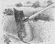
Illustrated is the Model D, with one rake side, one scraping side, and hoe tip, moulding potatoes.
