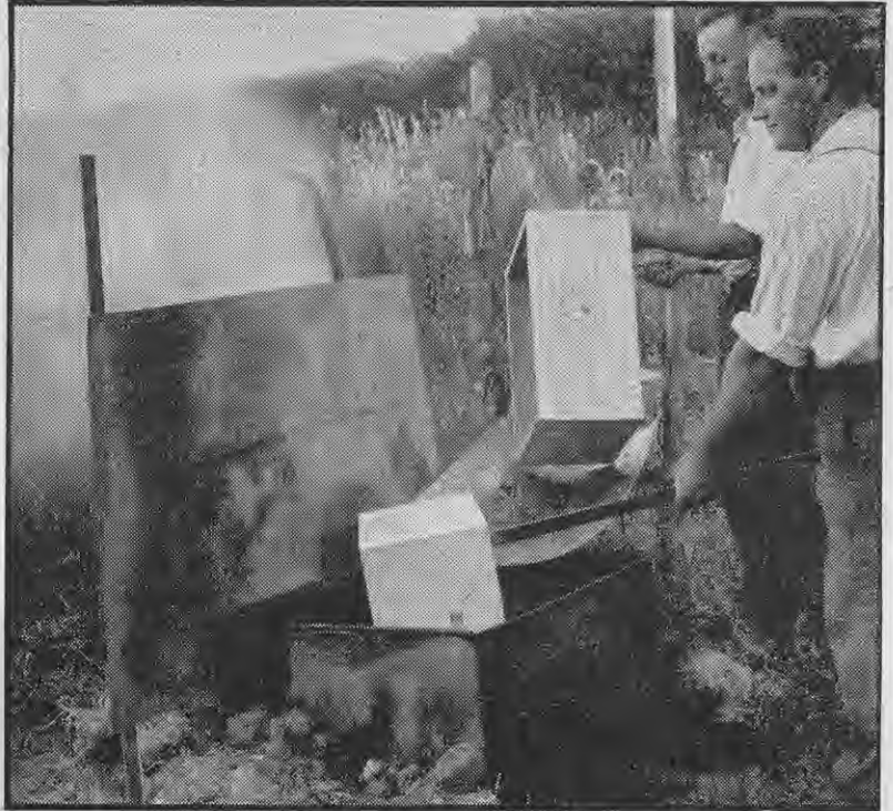
Hive parts being dipped in paraffin wax and drained. A protective shield may be seen at the back of the trough.
