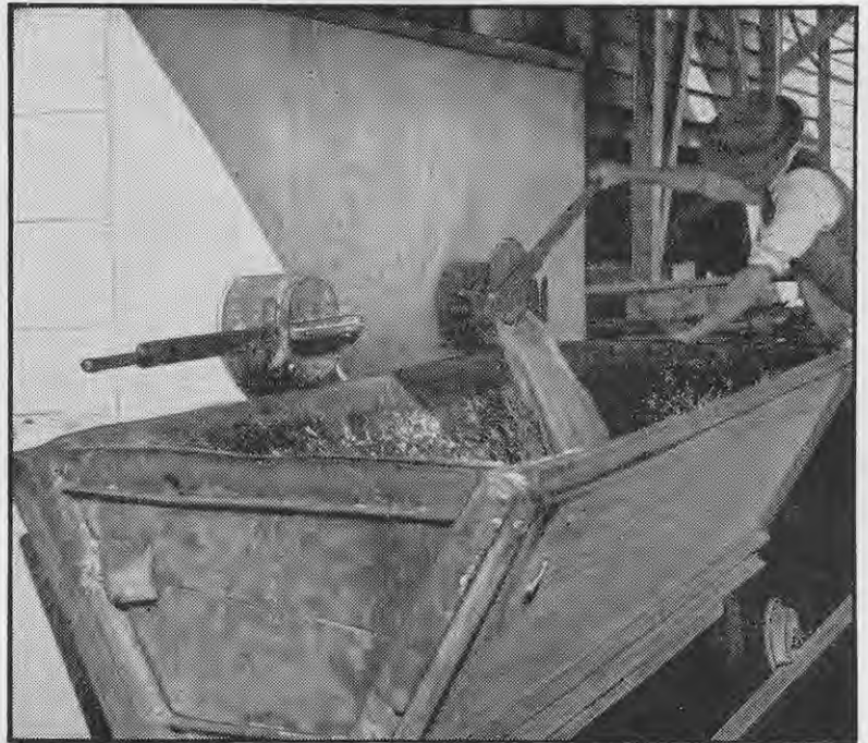
Releasing treated garbage into feeding trolley. The release valves are of a guillotine type capable of breaking bones.
