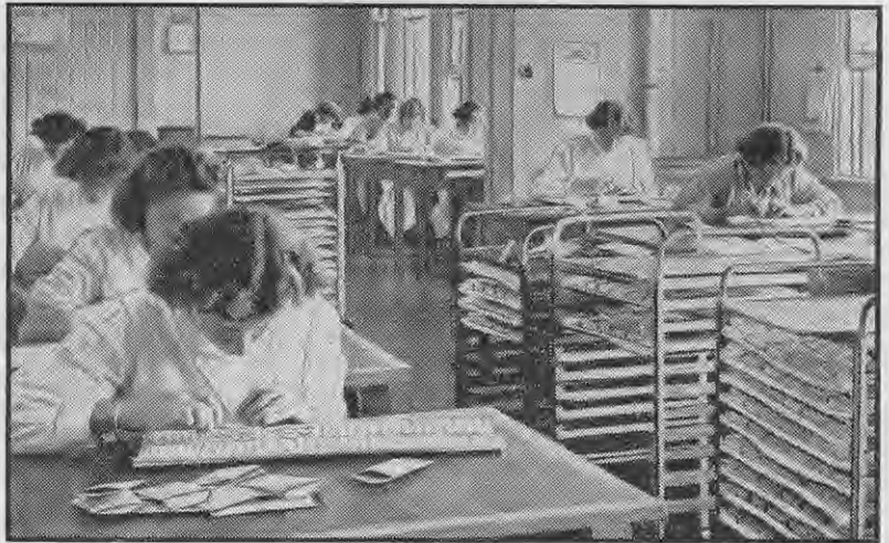
Counts being carried out in the germination laboratory. It is essential to know the exact germination when buying or sowing seed.
