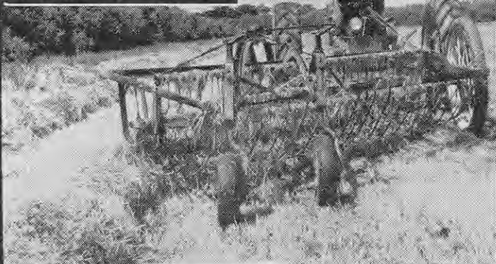
Modern 4-bar swath turner prepares crop for easier pick-up by forage harvester.
