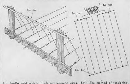
Fig. 3—The grid system of placing warming wires. Left—The method of tensioning. Right—Plan of the system.
