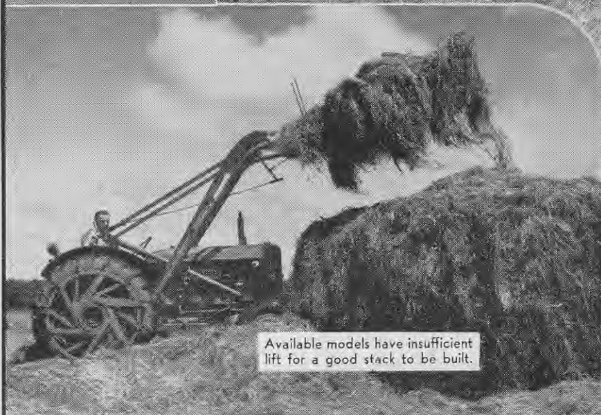
The fore-end loader picked up fairly well from swath and carried a good load.
