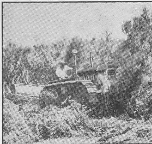
Heavy scrub is best crushed by a tracklaying tractor with scrub bar and heavy roller with steel flanges. A length of railway iron or a heavy swamp harrow with the spikes turned up serves to flatten light scrub for obtaining an efficient burn.
