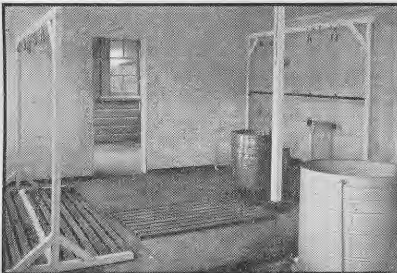
A poultry-killing room, with tanks of hot water for semi-scalding and cold water for cooling the birds. The birds are hung on the hooks on the right for sticking and bleeding and on those on the left for wet plucking.
