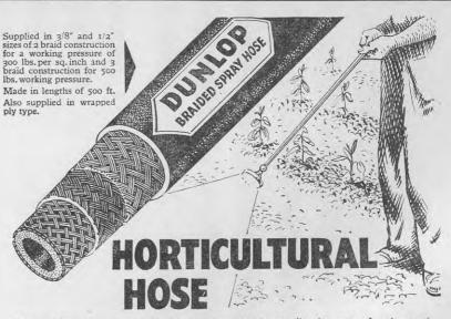
The modern high pressure power pump spray entails the use of a hose of exceptionally high quality and strength and Dunlop spray hose has been specially designed for this service. The rubber compounds used in the hose have been developed to meet the special conditions, the lining rubber being highly resistant to the chemical solutions used in spraying, whilst the cover
