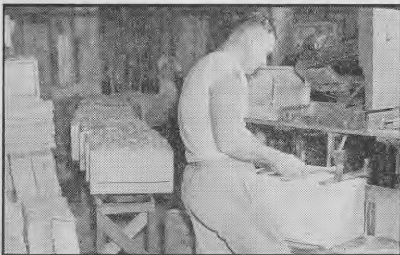
[National Publicity Studios photo.] Nails must be driven in straight, otherwise they may protrude either on the outside or inside of the case, making it dangerous to handle or damaging the fruit.
