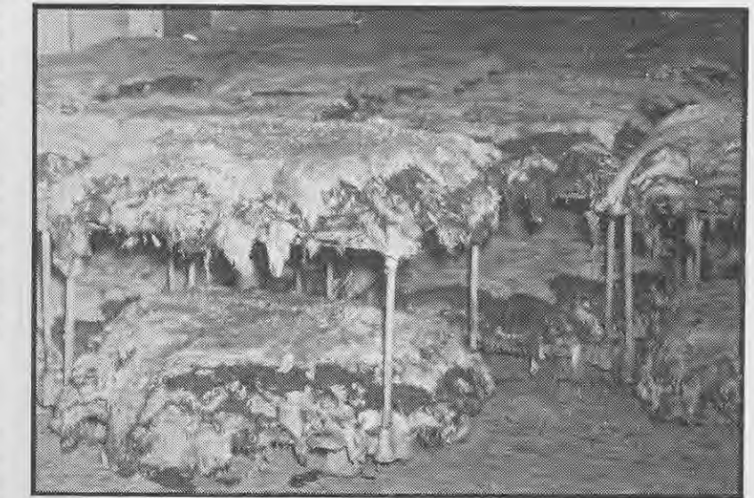
One method of stacking painted skins before pulling of the wool.
