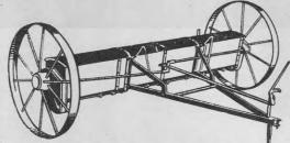
Designed to sow concentrated fertilizers in small quantities, as well as large applications of lime. (Has been successfully used for grass-seed sowing.) Rate of sowing varied from 35lbs. to 4000lbs. per acre. "Gates" can be set to any one of 16 different positions giving spraying action for thorough even coverage. Gears totally enclosed and protected. Call and see this machine or write for fullest details.
