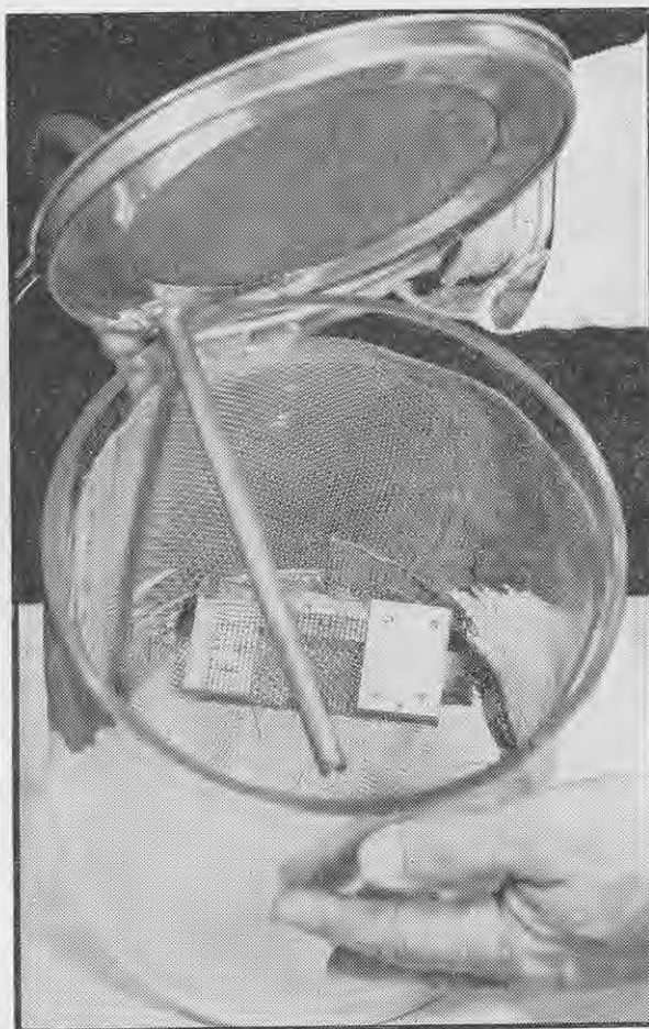
Fig. 5—A closer view of the container in which caged queens are treated with carbon dioxide.
