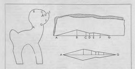
Making the head gusset. Left—The points where the width of the gusset will be changed are lettered on the side view. Upper right—These marks are transferred to the fold of a piece of paper the correct distance apart. Perpendicular lines half the width of the gusset are drawn from them and their ends joined. The gusset is then cut out of the folded paper. Lower right—A finished gusset, the points of which may be rounded.
