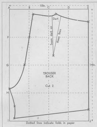
Take a piece of paper 10in. x 14in. Fold it in four lengthwise then again in four crosswise. Open the paper out and, using the creases as a guide, make pencil crosses at the following points:
