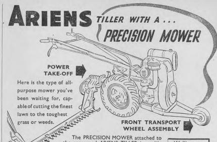
the PRECISION MOWER attached to the renowned ARIENS TILLER is readily adaptable to any terrain, the 42" wide cutting bar is easily set to cut from I"-1\frac{3}{2}" or 2\frac{1}{2}" high. The detachable front wheel gives a greater guiding control. For further information of this all-purpose combine, write to your nearest office of—
