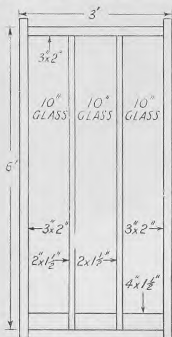
Diagrams of a frame 6ft. x 3ft. which will accommodate 5000 seedlings pricked out \frac{1}{2} in. apart in rows 1 in. apart or 2500 seedlings at 1 in. apart.
