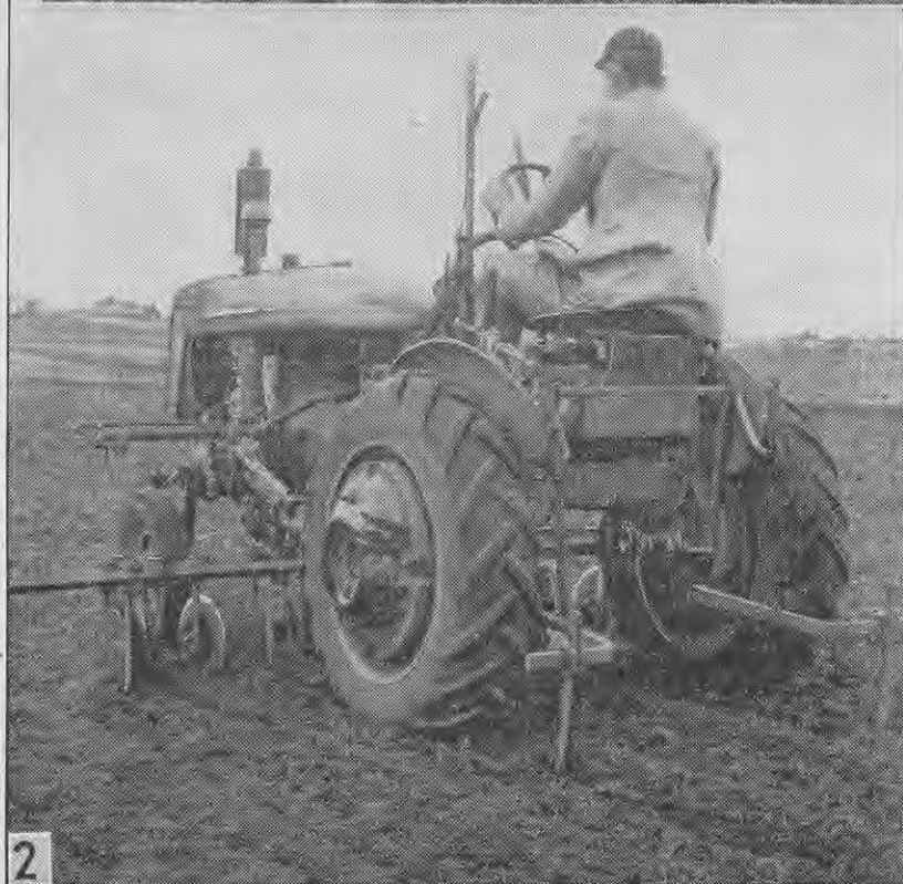
Upper—A 4-row seeder. Lower—A light tractor fitted with tractor inter-row cultivating equipment.
