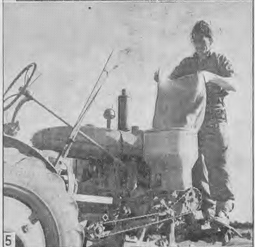
Upper—Front view of a light tractor equipped with knife weeders. Lower—Filling one of the two fertiliser bins attached to the tractor.
