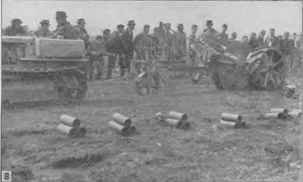
7. The Lewis drain digger. The vertical pair of discs cut into the ground, the cut section being picked up between the discs and carried over the top for discharge on to the rotary horizontal disc which carries the spoil well clear of the machine and tractor. 8. The Lewis digger in action. A cut 6in. to 8in. deep is made with each run; the front wheel enters the ditch and regulates the depth of the second and subsequent cuts.
