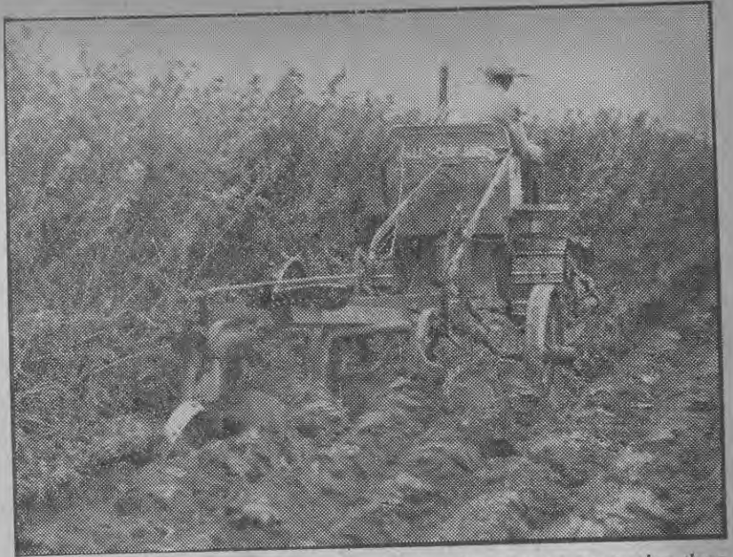
Sweet clover being ploughed in with a 35 h.p. kerosene tractor turning three 16in. furrows.
