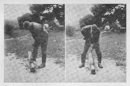
Edged tools are apt to be dangerous. An adze or a hand grubber is very liable to glance and cause serious injury if carelessly handled.
