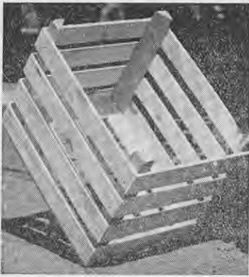
Specially designed onion storage crate made of pinus insignis and used in the heat storage trials.
