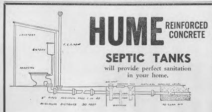
Why hesitate to obtain this necessary amenity when the cost is no more than that of connecting up with a sewer. In actual operation, the Hume Septic Tank is decidedly satisfactory, and is easily installed.
