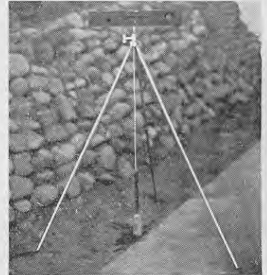
Fig. 4.—Level fitted to tripod for sighting to measuring pole.
